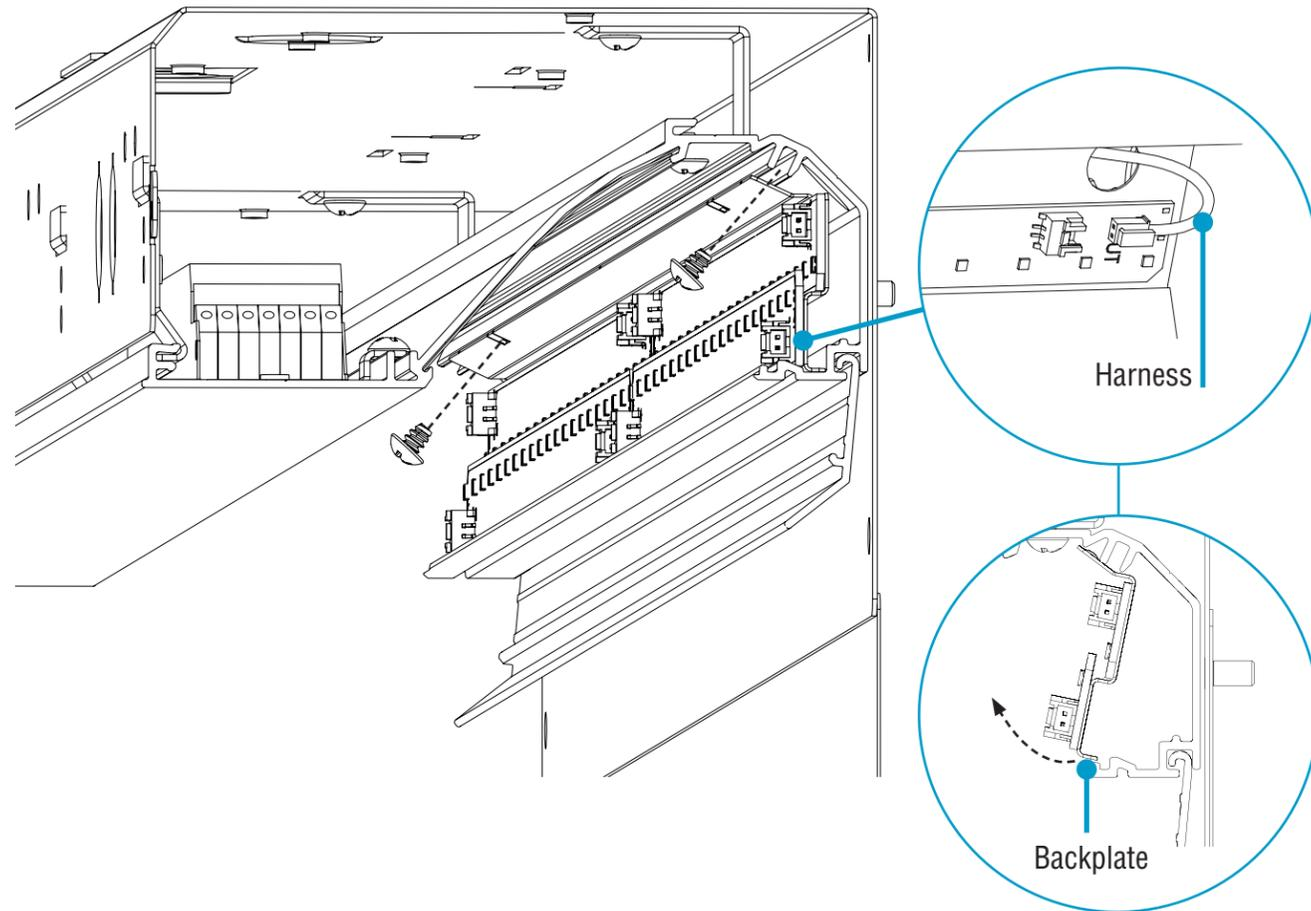
Remove two #8-18 x 1/4" screws that hold the backplate to carrier. Unplug harness and shunt. Keep shunt to put on the new LED board.
