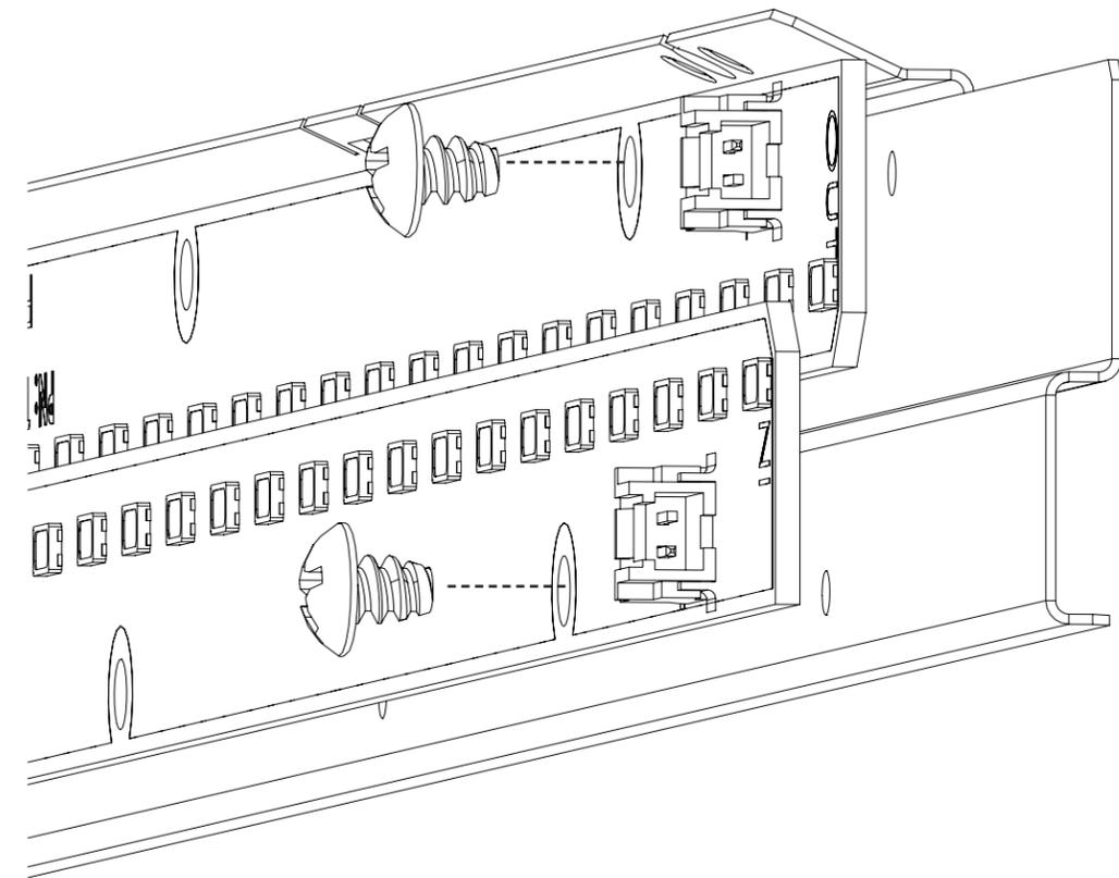
Remove #8-18 x 1/4" screws from LED board and install new LED board. Reconnect wiring and reinstall carrier by hooking to the luminaire housing brackets and securing with #8-18 x 1/4" screw. **Reinstall diffuser and turn power on to luminaire.**
