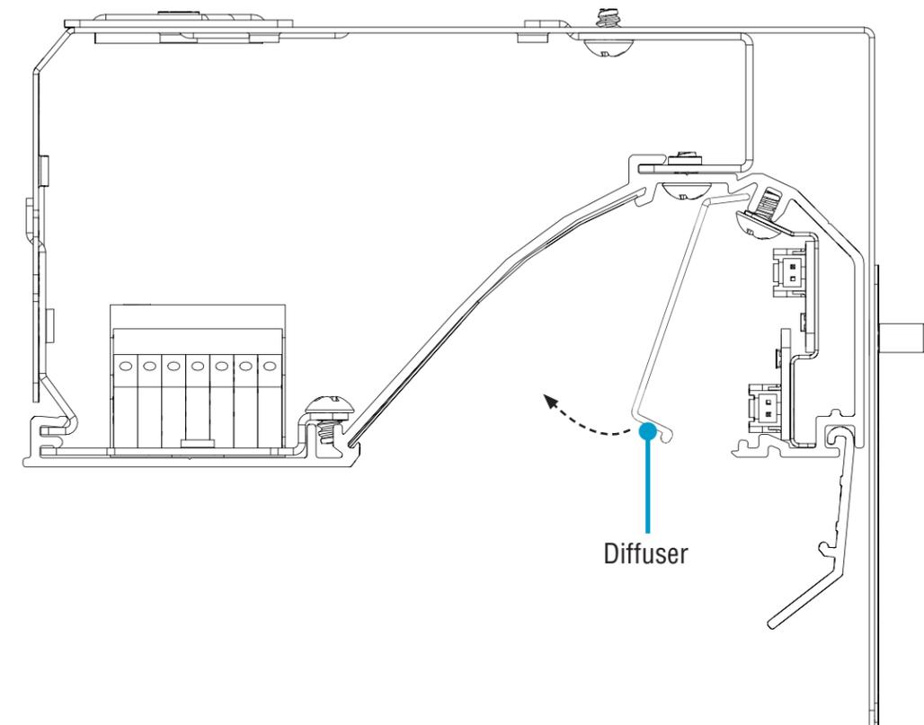
Unsnap the diffuser to remove it from the luminaire. We recommend using a putty knife. Set diffuser aside to prevent from getting or damaged.
