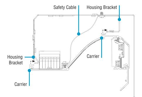
B. Secure Carrier & Snap Kickplate Side View
