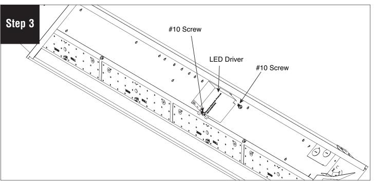
Remove 2 #10 screws that hold the driver, and disconnect all electrical connections. Remove and replace new driver. Reconnect all electrical connections and reinstall driver cover and lens.
