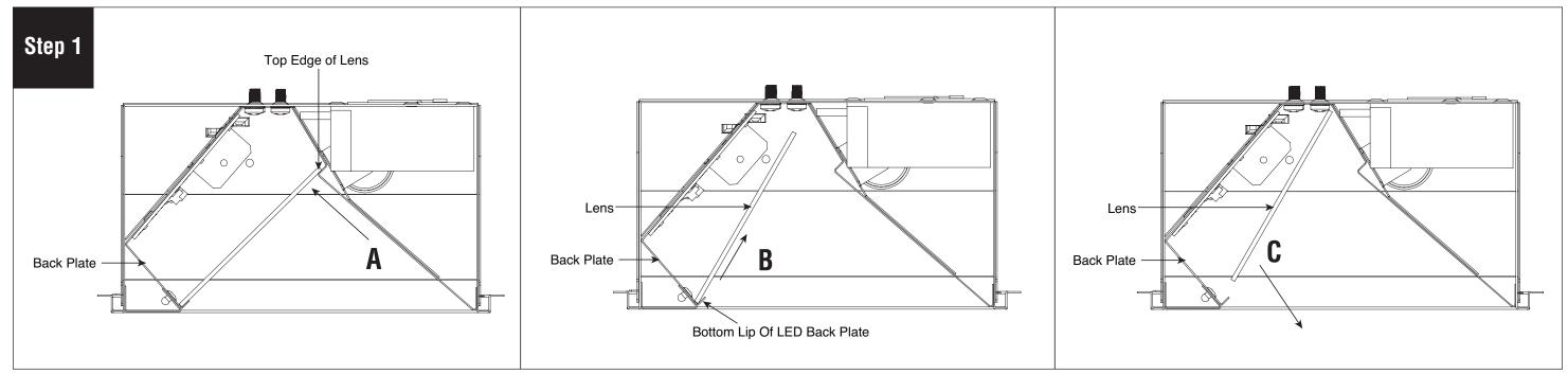
A. Remove the lens by pushing the top edge of the lens in. B. Lift the lens up slightly to clear the bottom lip of the led back plate. C. Then swing the bottom edge of lens away from back plate. Set lens aside.
