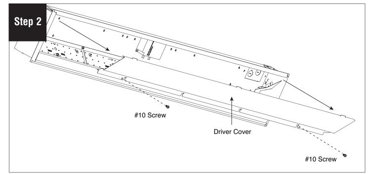
Remove 2 #10 screws. Then remove driver cover.
