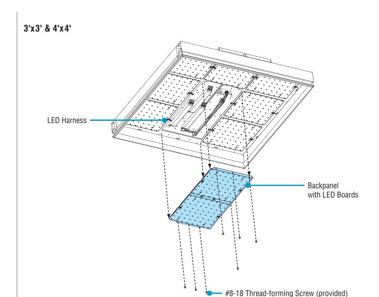
• Remove backpanel with LED boards by removing the #8-18 thread-forming screws.
