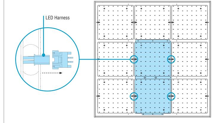
• Replace backpanel with LED boards by replacing the #8-18 thread-forming screws.
