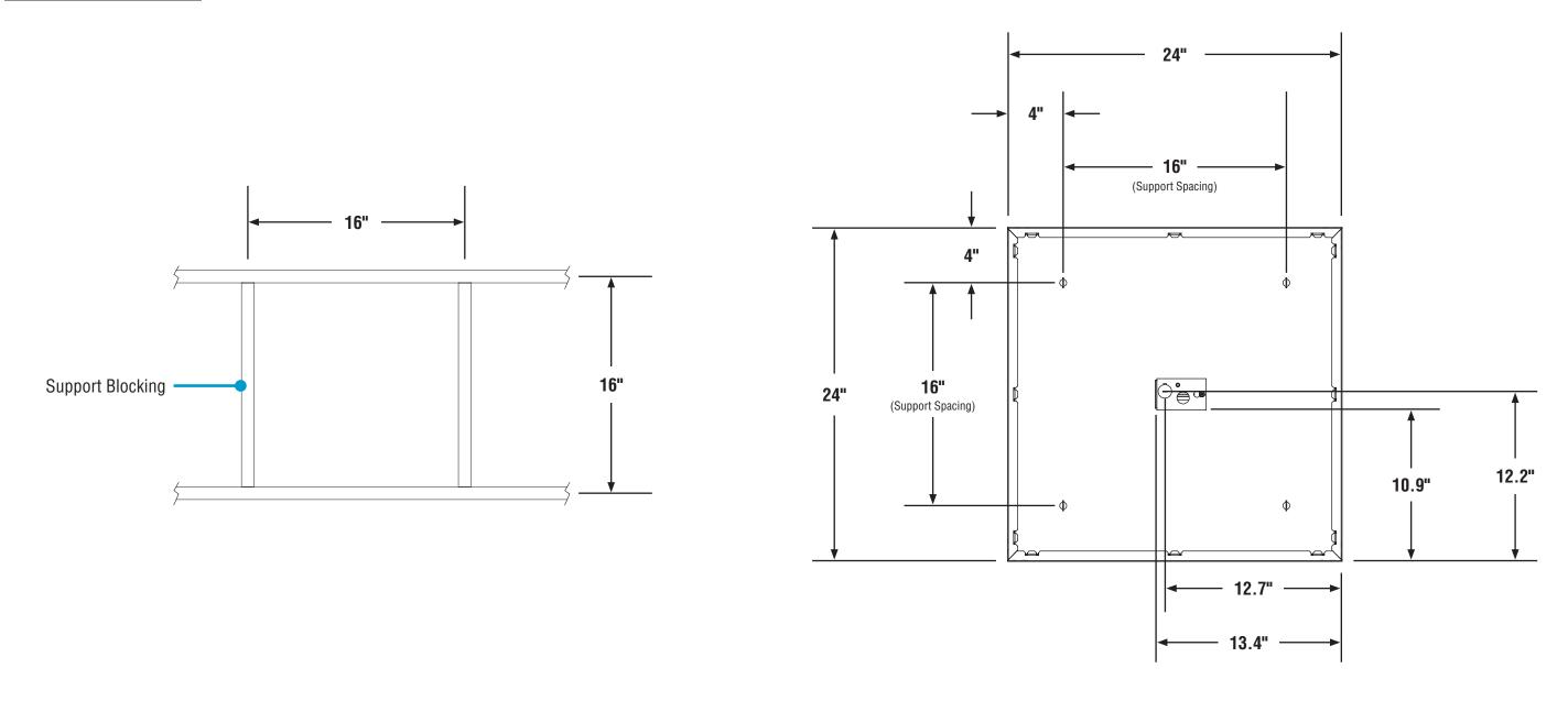
• Luminaire mounting holes sized for 1/4"-20 hardware.
