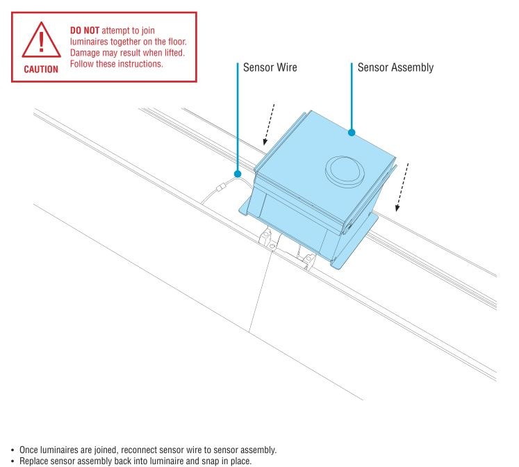
Once sensor is in place, refer back to Luminaire Installation Instructions: Closing Luminaires.
