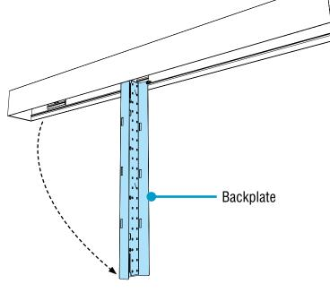
• Carefully rotate backplate out and let it hang from luminaire body.
