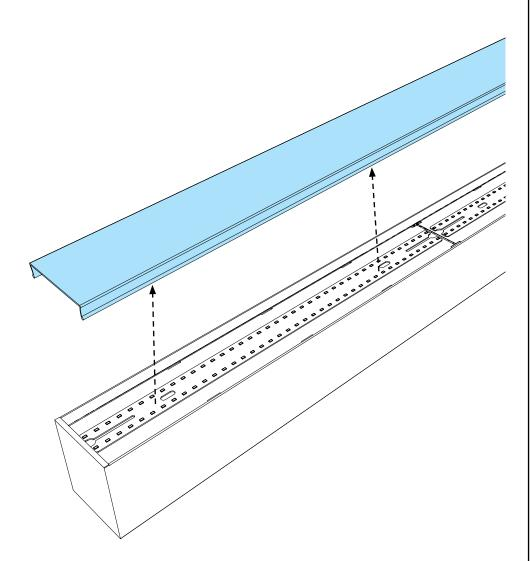
· Remove diffuser and set aside to prevent from getting dirty or damaged
