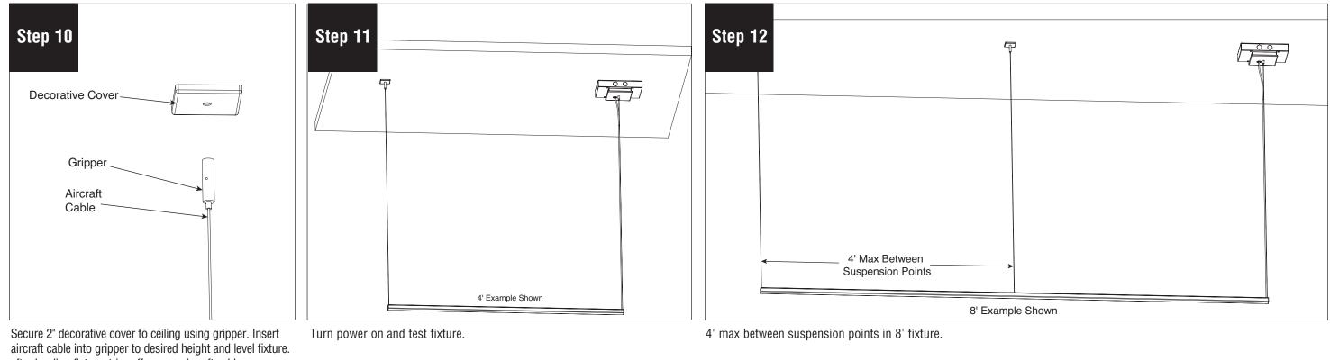
after leveling fixture, trim off excess aircraft cable.
