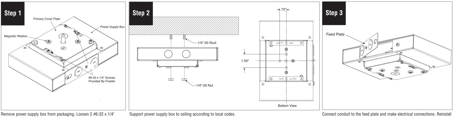
screws (provided) with #2 philips screw driver and rotate primary cover plate to remove.
