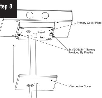
Use small knockout and add strain relief (provided) to single power cable. If multiple power cable, use large knockout and attach cable tie through center cross bar hole.
