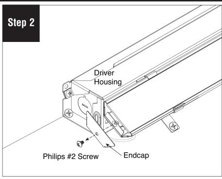
Remove Philips #2 screw on endcap using Philips screw driver.
