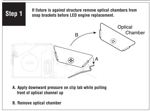
Confirm which LED engines need to be replaced. Shut off power to the fixture. Remove optical chamber from snap brackets (if fixture against structure).
