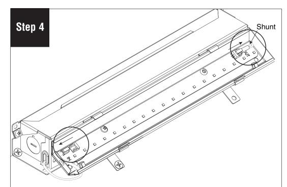
Carefully disconnect wire plugs from the LED engine. Be sure to retain the end shunt (wire loop) and re-use with new LED engine.
