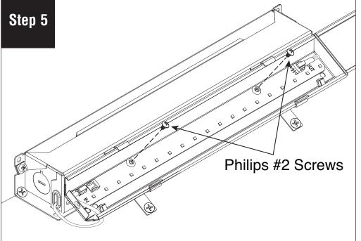
Remove Philips #2 screws securing the LED engines. Replace with new LED engines. Carefully reinstall screws. Avoid any contact with LEDs during this process!
