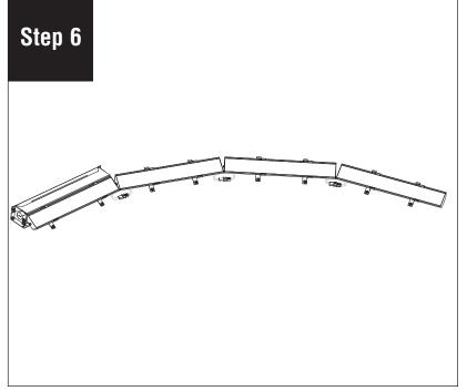
Reconnect all wires and end shunt connecting the same as originally wired. Reinstall lenses, close up the fixture and re-secure all screws that were removed.
