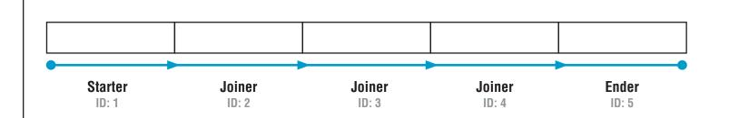
Hang luminaires in ID order. Hang prior to joining. Hang, level, join, repeat to the end of the run.
