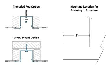
Two mounting options: threaded rod and screw mounting options. Mounting locations are located on each end of the luminaire. Mounting location is 4" away from each end of luminaire
