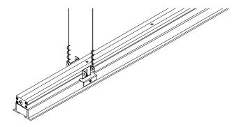
HPX-R for T-Bar installations comes standard with a splice plate at the end of the luminaire. Mounting brackets (supplied) secure the luminaire to T-Bar and provide support to structure location. All even foot length (2, 4, 6...) luminaire runs are reduced in length an appropriate amount to fit within typical 2×2 and 2×4 T-Bar grid systems. For uncommon T-Bar systems please consult factory.
