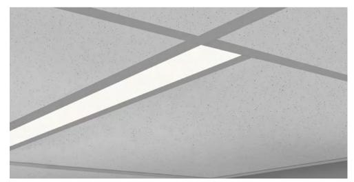
The High Performance 2.5" Aperture (HPX) is a patented LED linear luminaire with a square micro profile and internal driver design. This Line-of-Light luminaire delivers excellent performance and is equipped with a unique LED configuration for superior illumination. HPX can be tailored from 2' to 12' sections in 1' increments and is available in Pendant, Surface Mount, and Recessed.
