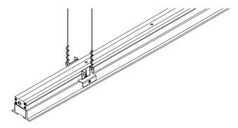
HPX-R for T-Bar installations comes standard with a splice plate at the end of the luminaire. Mounting brackets (supplied) secure the luminaire to T-Bar and provide support to structure location. All even foot length (2, 4, 6...) luminaire runs are reduced in length an appropriate amount to fit within typical 2×2 and 2×4 T-Bar grid systems. For uncommon T-Bar systems please consult factory.
