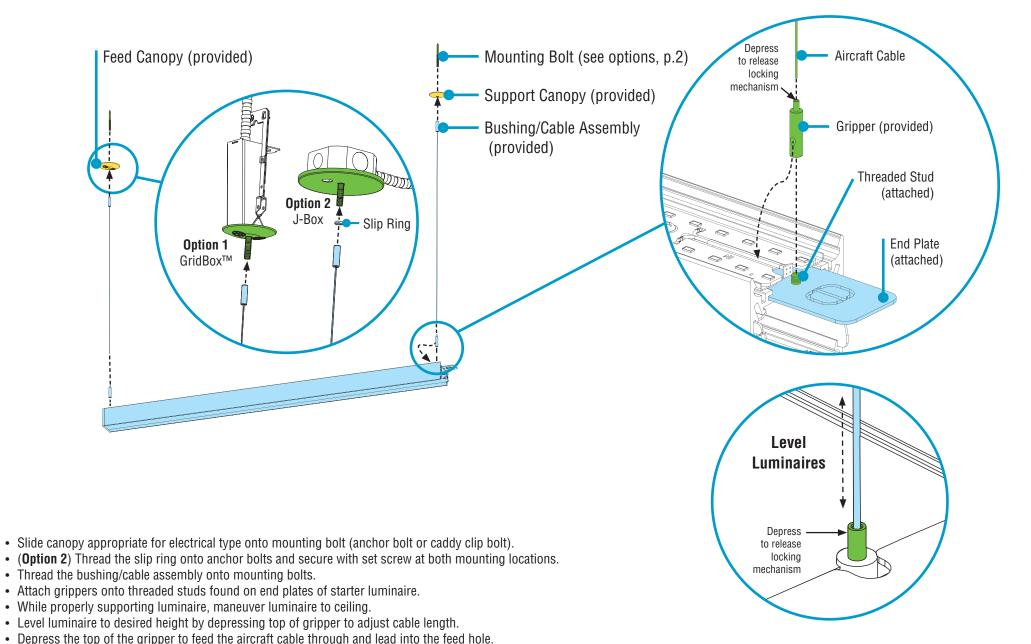
B. Make Electrical Connections Bottom-Up View
