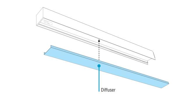
Reinstall backplates by inserting into luminaire body. Hear 4 clicks per LED backplate. Make sure ALL LED backplate secure before reinstall diffusers.
