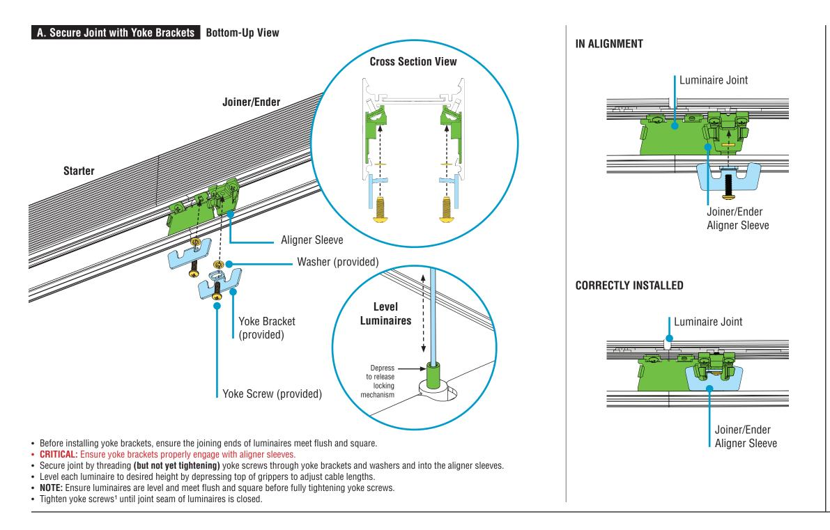
Yoke Bracket w/ Screw and Washer #10-32 x 5/8" (provided)
