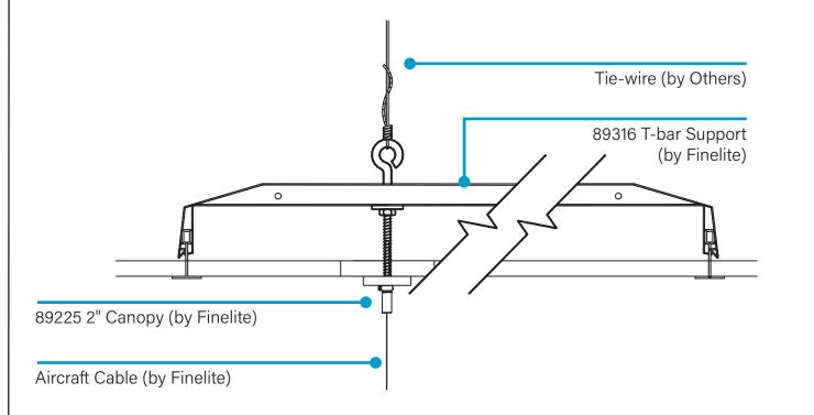
Non-power supports will be equipped with a 1/4 x 20 Eyebolt and a 2-inch canopy. All supports must be securely fastened to the structure using Tie-wire (supplied by others) in accordance with code regulations.
