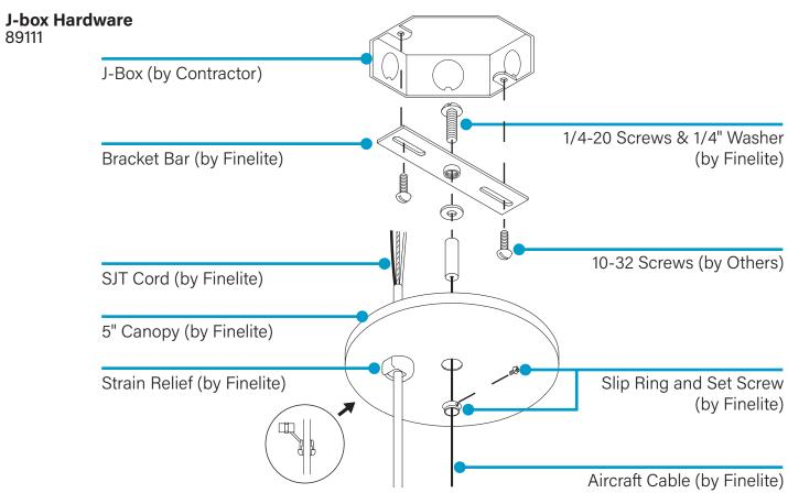
For off-grid mounting, utilize the Caddy 512 bar along with our C4-Jbox hardware. This combination allows the Caddy 512 to span two parallel T-bars, each 2 feet apart, and provides a suspension point in the middle of the ceiling tile. The power connection requires a J-box attached to the Caddy 512 bar, and our 5-inch canopy will be provided for the feed location.
