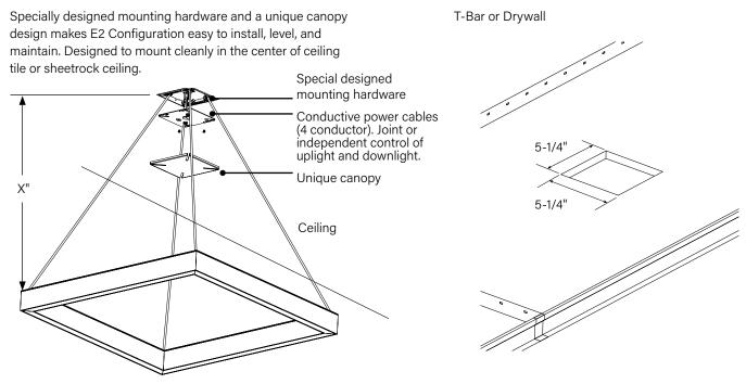
X" = Adjustable Power Cable length (18" or 24") from ceiling to luminaire.
