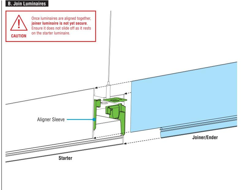
• Align joiner/ender luminaire with aligner sleeves on starter and slide together. Be careful not to damage any wiring.
