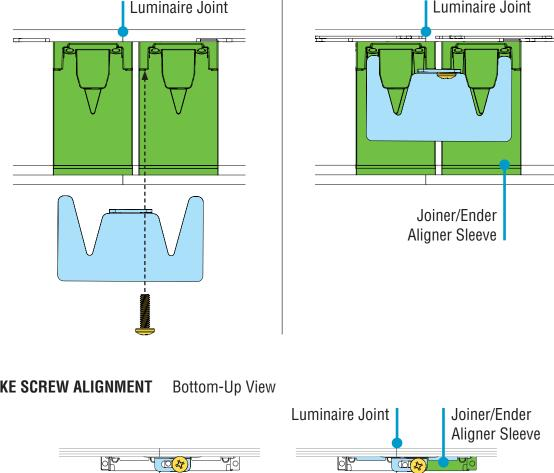
**NOTE:** Yoke screws should be installed directly across from each other, not diagonally, and in holes furthest from the joint line. One voke screw per one voke bracket.
