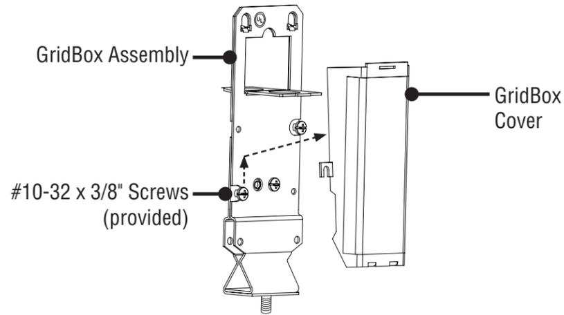
Loosen (2) #10-32 x 3/8" screws and temporarily remove the GridBox™ cover.
