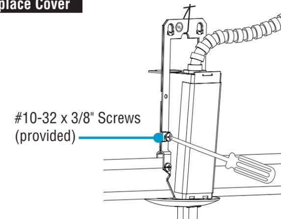
Arrange all wiring neatly towards the center of the assembly and place cover to align with mounting holes. Tighten (2) #10-32 x 3/8" screws until the cover is flush with the assembly. Make sure there are no pinched wires. Notch ceiling tile around the GridBox outline and install.
