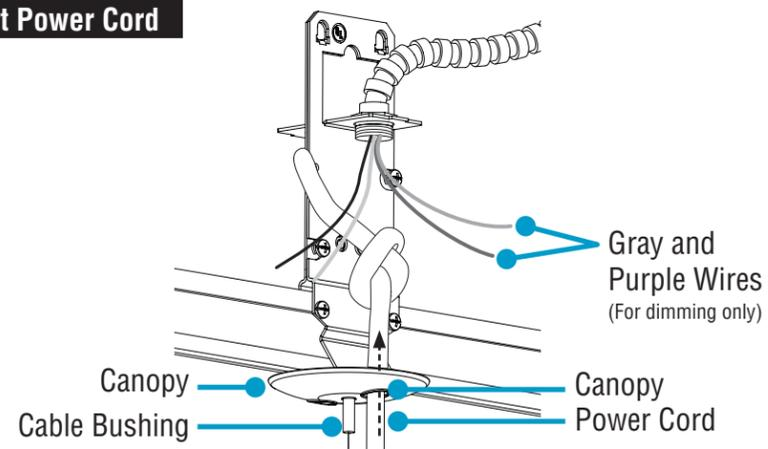
Insert luminaire power cord from luminaire through the bushing in the canopy. Align the canopy with the 1/4"-20 threaded stud on the GridBox assembly and screw on the supplied cable bushing which holds up the luminaire. Make sure it's finger tight and snug to the T-Bar. This may have to be repositioned after the ceiling tile is installed. **IMPORTANT:** Place an overhand strain relief knot on the cord.
