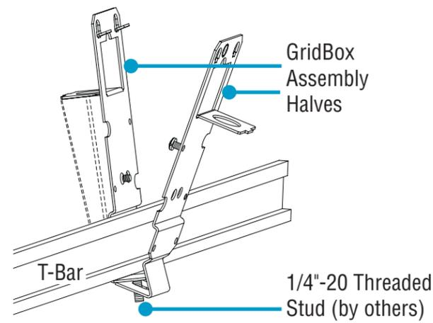
Separate the two halves. Rest the T-Bar on one half and guide the 1/4"-20 threaded stud at the bottom through the elongated slot of the other half. This stud is used to hold on the luminaire cable bushing.
