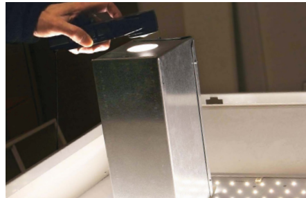
Color consistency is tested at the LED manufacturer and luminaire manufacturer.
