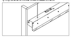
Allows a luminaire to be installed after ceiling framing is complete.
