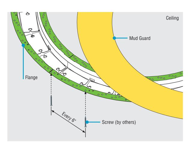
Secure flanges to ceiling using appropriate screws or fasteners<sup>1</sup> for hard surface, per local building codes.
