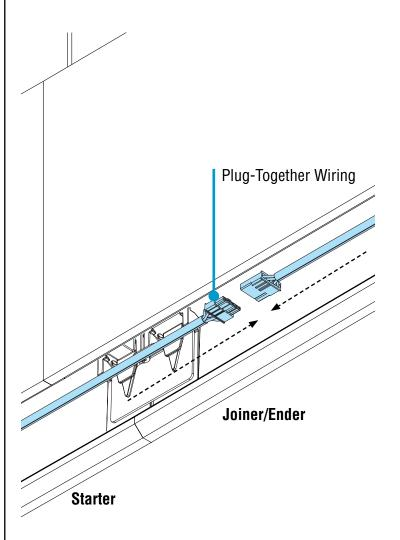
• Connect plug-together wiring.
