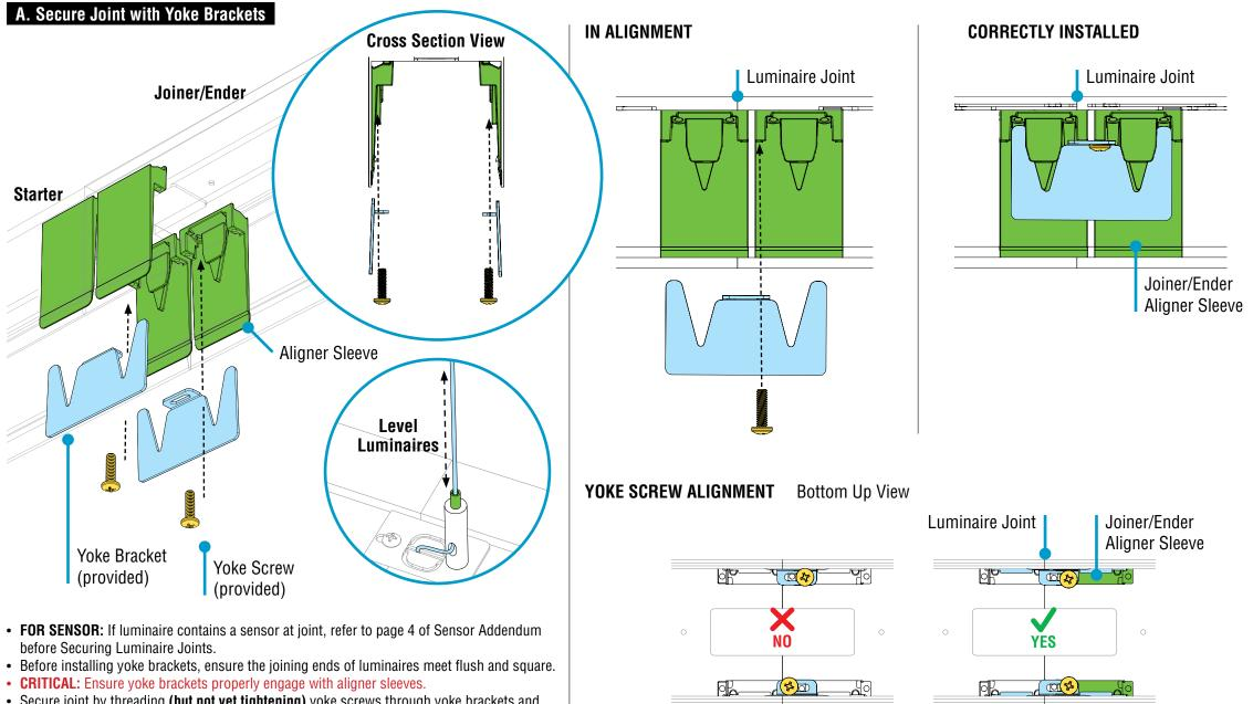
• Secure joint by threading (but not yet tightening) yoke screws through yoke brackets and into the aligner sleeves.
