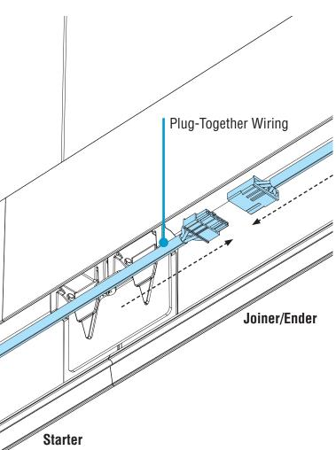
• Connect plug-together wiring.
