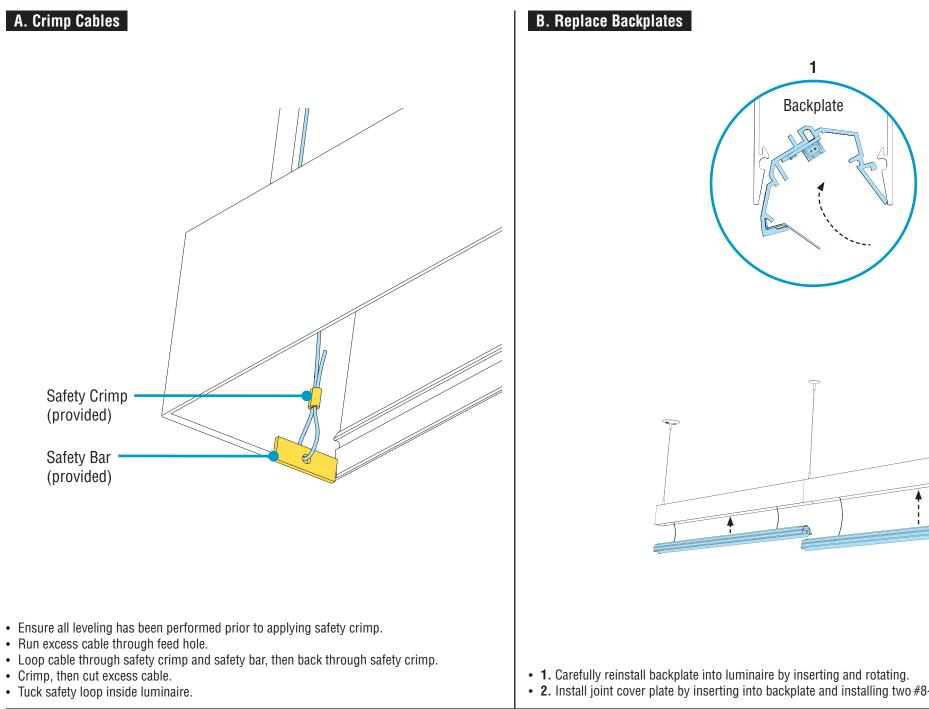
• Ensure all leveling has been performed prior to applying safety crimp.
