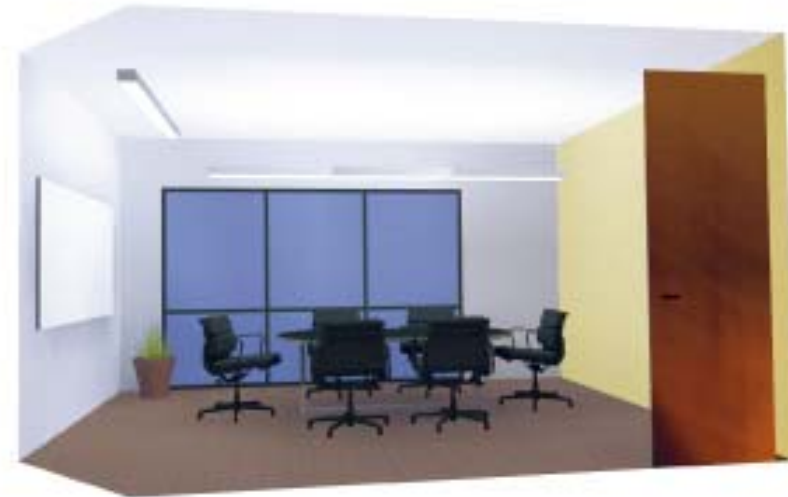
Figure 7. A streamlined approach for conference rooms using indirect/direct lighting for general and AV modes plus a separately controlled whiteboard luminaire provides ideal functionality for all uses of the room and low energy use
