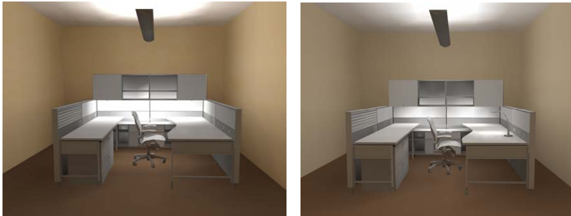
Figure 5. Reduced overhead lighting with fluorescent task lighting results in high contrast ratios with an over-lit work plane (left), while reduced overhead lighting combined with LED task lighting promises balanced lighting at a low power density (right).
