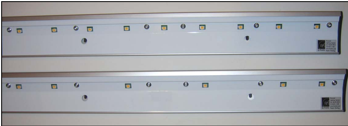
Figure 14. The 6 and 9 Watt undercabinet luminaires were designed to use the same frame and circuit board, with 3 LEDs omitted in the 6 Watt version.
