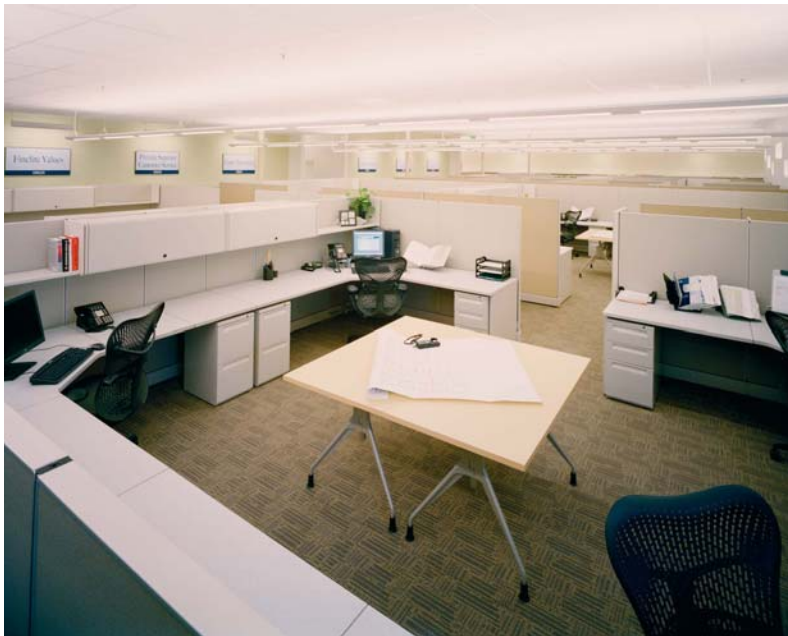
Figure 1. Uniformity and balance are key to achieving a low level ambient system at target levels of 0.5 to 0.65 watts per square foot.
