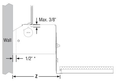
\* Gasket provided by Finelite goes into this 1/2" gap between the luminaire and the wall
