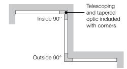
Fully illuminated 90° corners with telescoping and tapered optics standard. Consult technical sheet for telescoping lengths on inside and outside corners.
