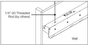
2 Install luminaire onto 1/4"-20 threaded rod (by others).
