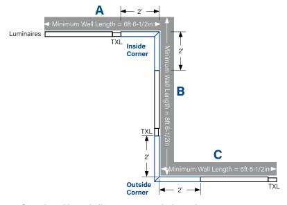
Configuration with pre-built 90° corners and telescoping\*
