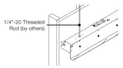
Allows a luminaire to be installed after ceiling framing is complete.
