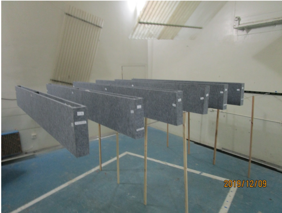
Figure 1 – Specimen mounted in test chamber
