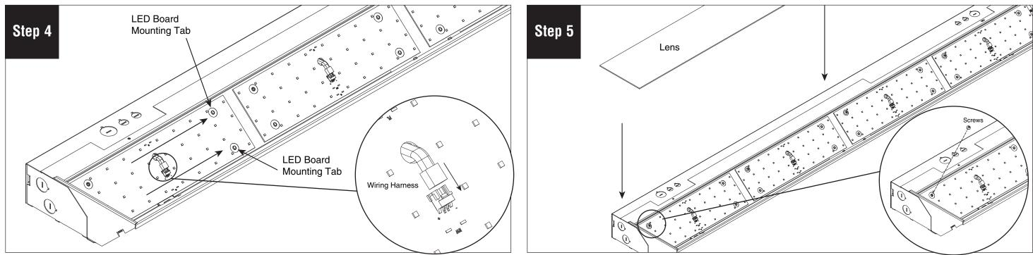
Slide LED board toward the mounting tab. Reconnect LED wiring harness.
