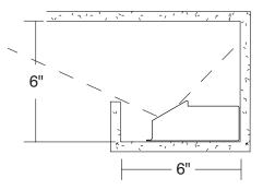
Designed to fit into an architectural cove with a suggested cross section of 6" x 6" or larger.
